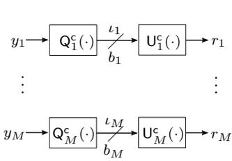
Fig. 2.(a) Conventional ADC Unit
