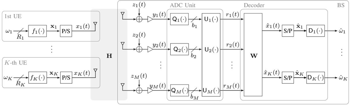
Fig. 1. ADC-Constrained System Model.
