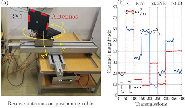
Fig. 2. (a) Receiver RX1 located on 5<sup>th</sup> floor of the Institute of Telecommunications at Vienna University of Technology. (b) Example of the estimated outdoor to indoor channel  $|\hat{\mathbf{H}}_{11}|$  (blue solid line) and indoor to indoor channel  $|\hat{\mathbf{H}}_{13}|$  (red dashed line) computed from each received frame.
