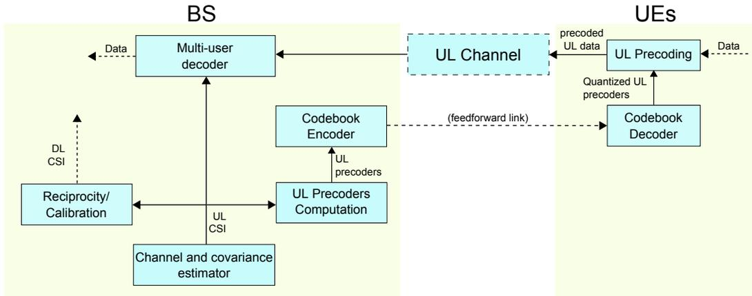
Fig. 2. Functional block diagram of the single-cell system considered in the simulation.
