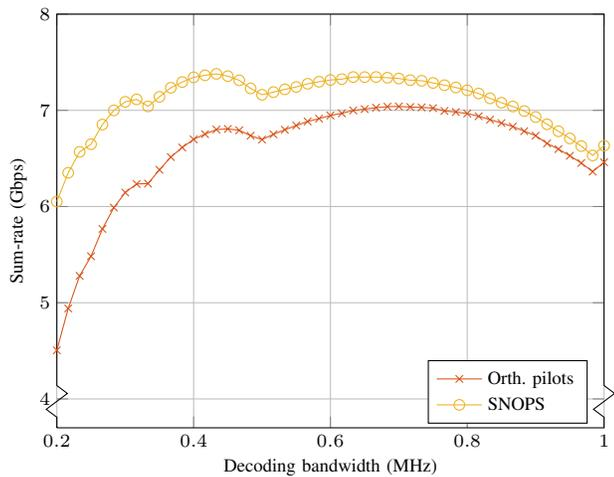
Fig. 4. Comparison of the sum-rate achieved with full pilots and shorter, non-orthogonal pilots from [19]. We consider different granularities of decoding bandwidth, with sounding efficiency factored in.
