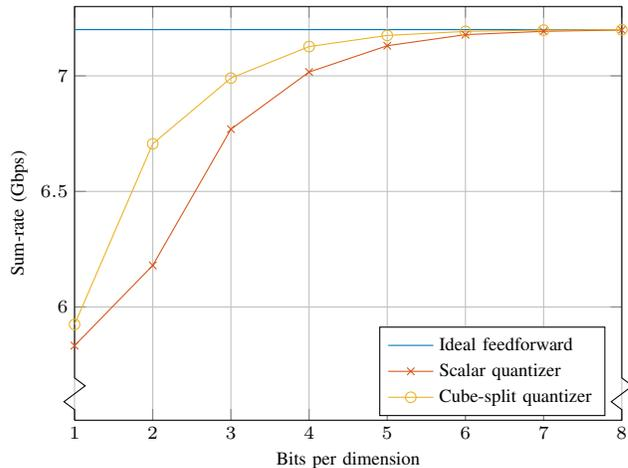
Fig. 5. Performance of the feedforward quantizers, comparing the cube-split quantizer [29] with a baseline scalar quantizer with a similar number of bits per dimension.
