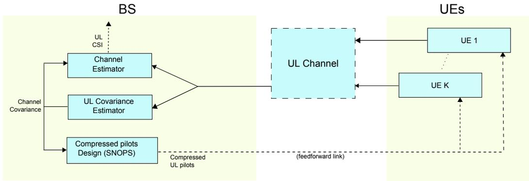
Fig. 1. Block diagram of a Covariance-Based CSI acquisition system.
